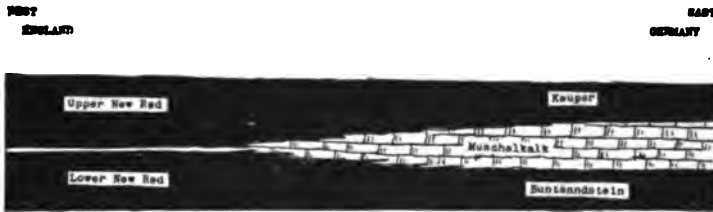
FIG. 1594. — Diagrammatic section (ideal), showing the east-west relationship of the Triassic strata in northern Europe. In England the series comprises red sandstones throughout (New Red Sandstone), in Germany the threefold division into Buntsandstein, Muschelkalk, and Keuper is typically developed. (Original.)
